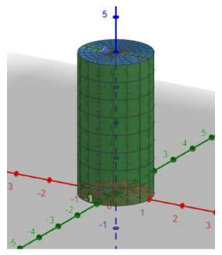
We are integrating over the region S which is part of a solid cylinder, thus we change to cylindrical coordinates to do the integral (which is just polar coordinates plus a z coordinate).
